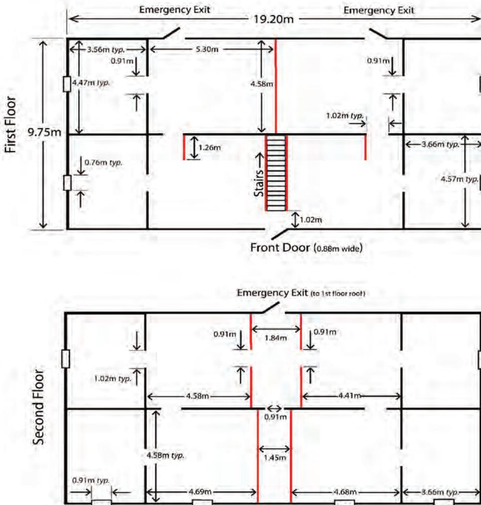
Figure C-2: Dimensions of the Burn Prop Floor Plan
