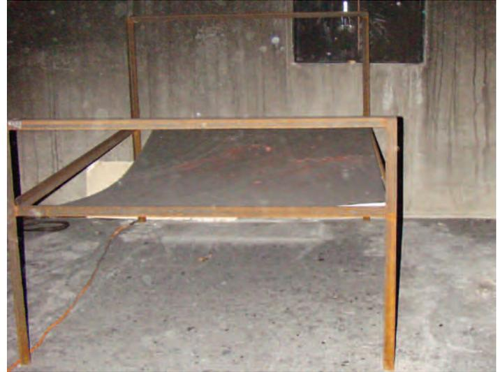
Figure 5: Noncombustible Furniture Used in the Time-to-Task Experiments
