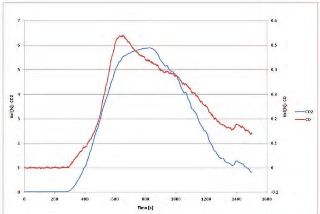
Figure 39: Representative Carbon Monoxide and Carbon Dioxide Concentrations
