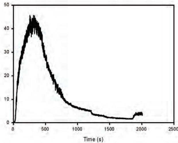
Figure A-13. Temperature, Gas Concentration, and Heat Flux During Test CRA 3, 4 Pallets, Fast Ignition Scenario
