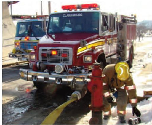
Figure 16: Connecting to the Hydrant
