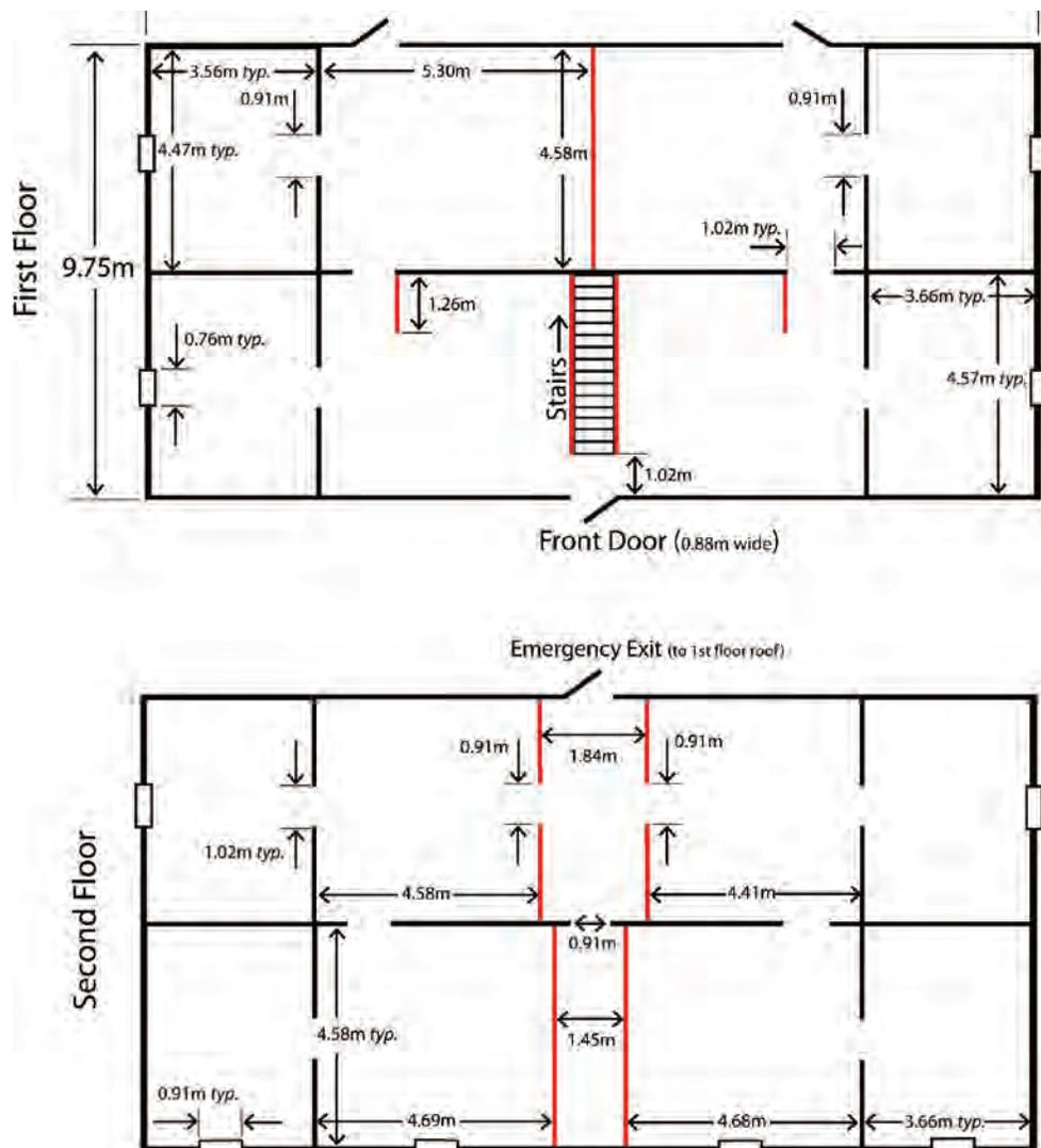
Figure 4: Dimensions of the Burn Prop Floor Plan
