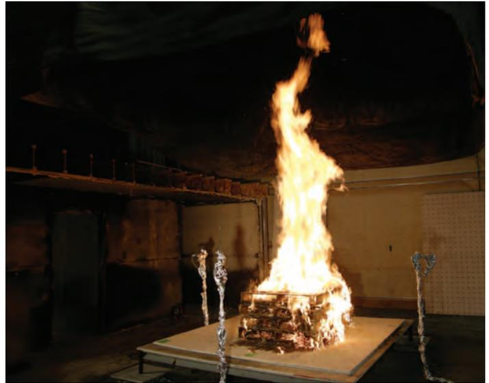
**Figure 2: Test Burn of Pallets in Laboratory**
